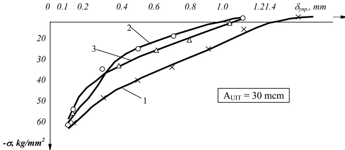
**Fig. 4. Residual stress values in a surface layer at different treatment speeds**
