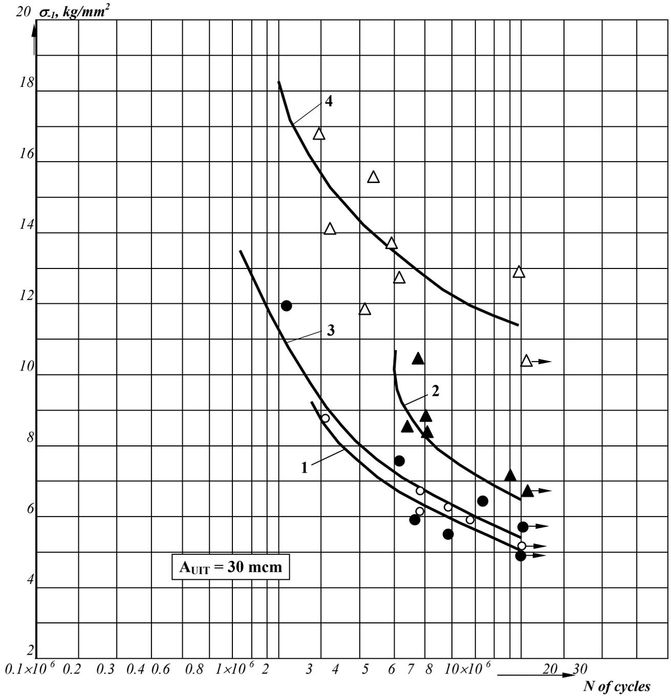
**Fig. 7 Corrosion-fatigue strength of samples:**
