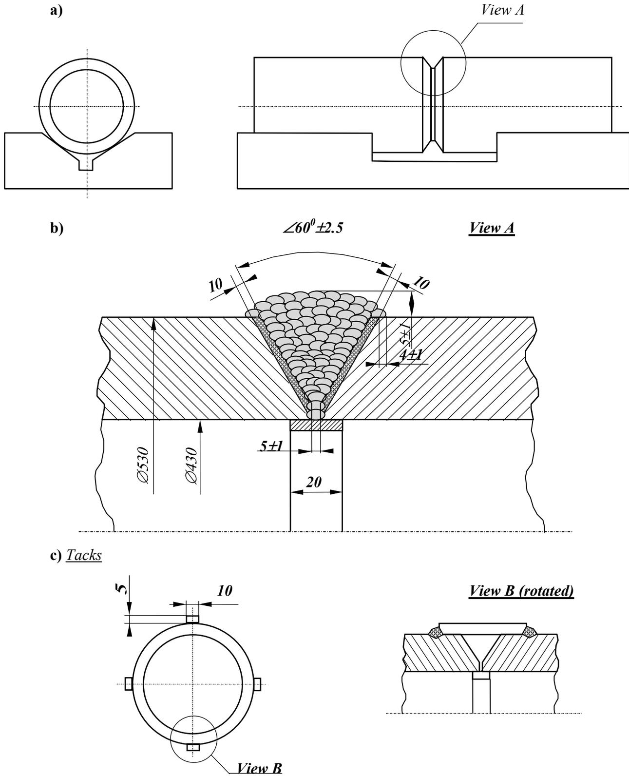
**Fig. 2 Setup for UIT Testing**
