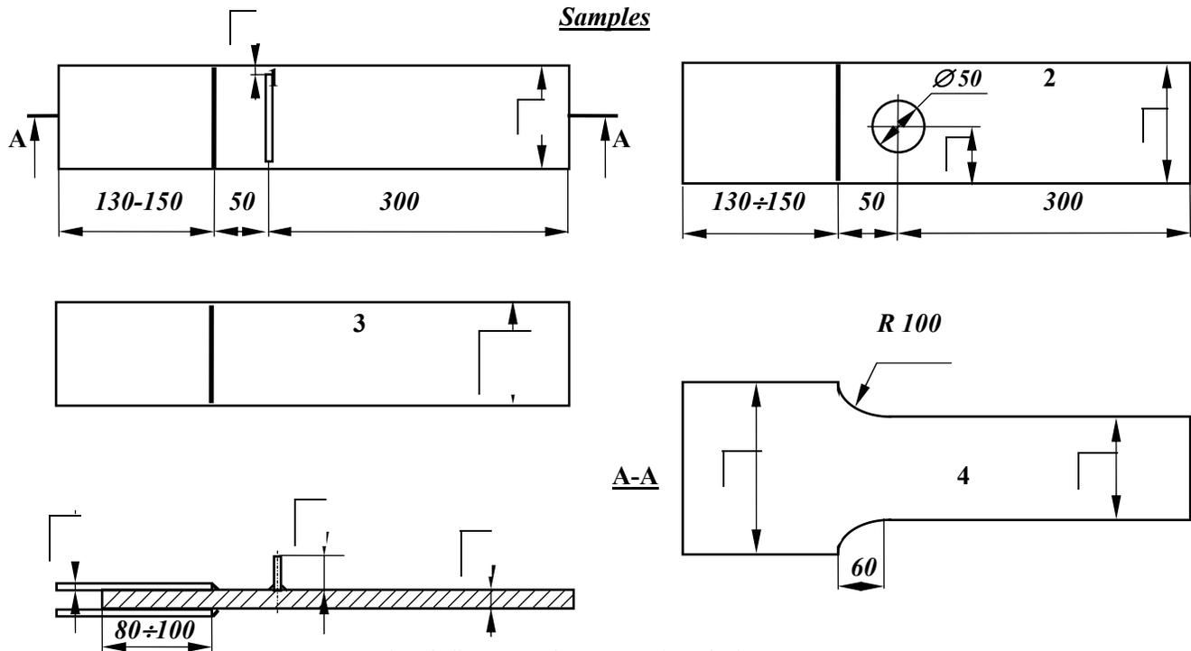
**Fig. 6. Samples for corrosion-fatigue tests**
