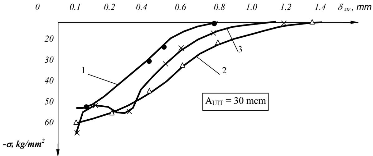
**Fig. 5. Intensity of metal strengthening that had been in use at various treatment speeds:
