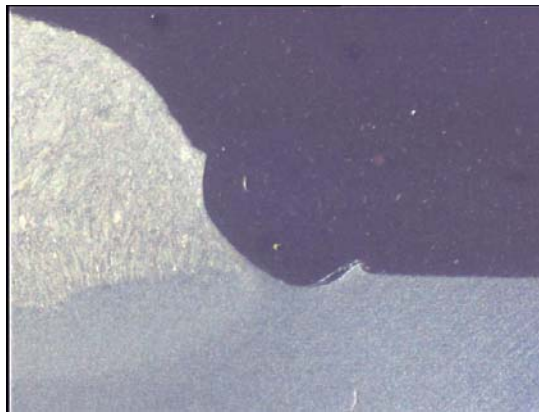
Figure 12 – Example of S355 weld shape after UIT (toe radius = 0.90mm, undercut depth = 0.4mm)
